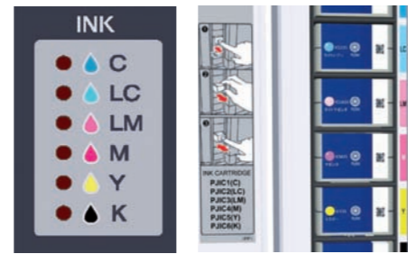
The ink cartridge for each colour can be easily changed in just a few seconds
